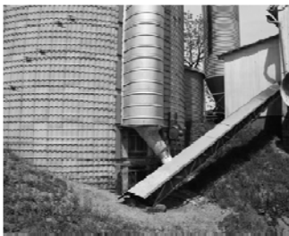
Prepare for flare ups. Observe from loading platform and bottom of chute with charged lines.
