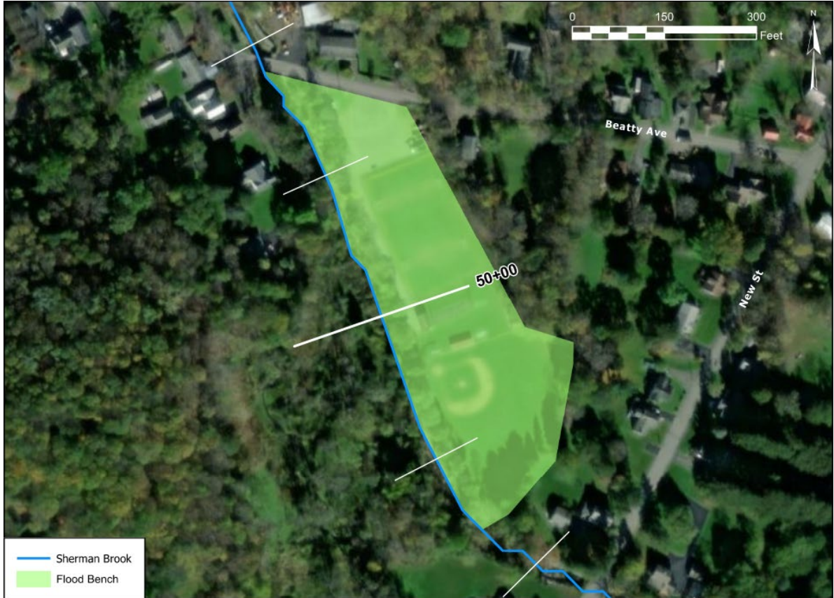
Figure 7-9. Placement of proposed flood bench at High-Risk Area #3 along Sherman Brook.
