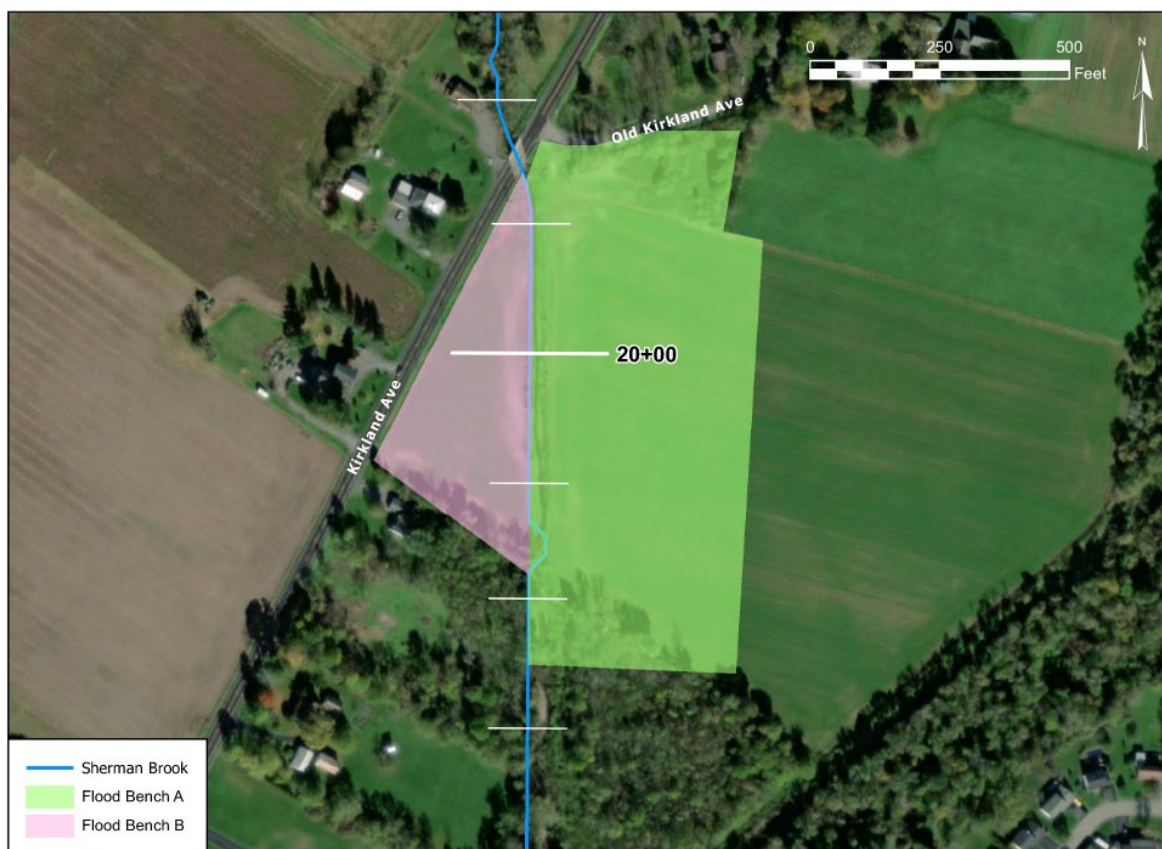
Figure 7-28. Placement of proposed flood benches at High-Risk Area #5 along Sherman Brook.
