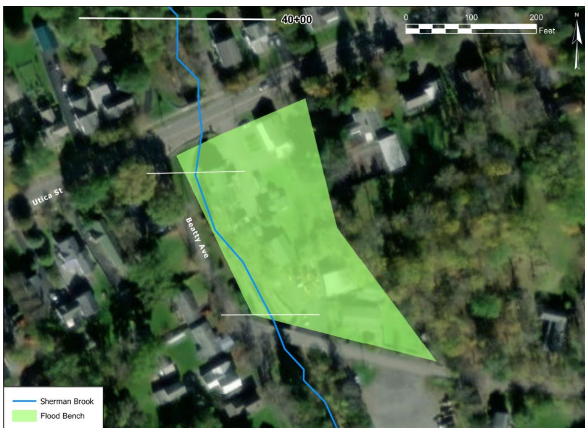
Figure 7-18. Placement of proposed flood bench at High-Risk Area #4 along Sherman Brook.
