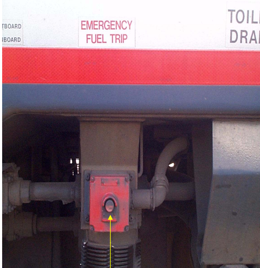
Emergency Fuel Trips (shut offs) on each side of the locomotive.
